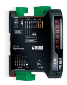
High-performance multifunctional weight transmitter, the fastest of the Dini Argeo range. It can manage up to 4800 readings per second, for weighing with precision in milliseconds. For DIN rail mounting, it allows direct reading and diagnostics of the connected weighing system. The wide range of available interfaces makes the integration of weighing into any automation system easier and safer.
